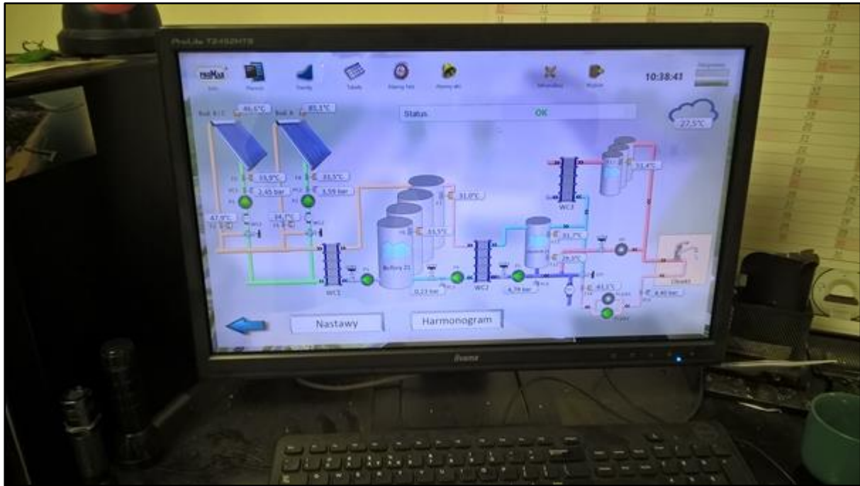
Figure 12 Control SW for solar heating system in the public hospital in Kolobrzeg
